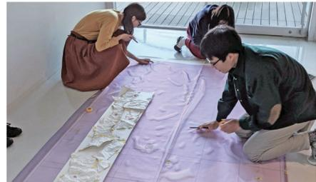
Transferring the 1:5 scaled cutting pattern to the cloth roll, using grid for enlargement
